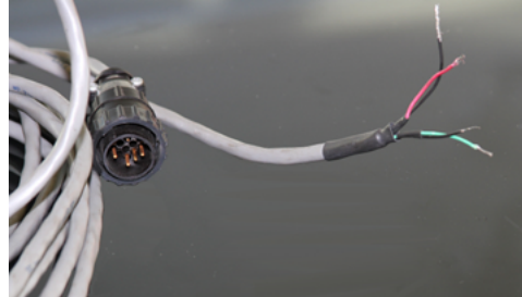
This CNC Interface cable has two pairs of wires: red / black and green / black
